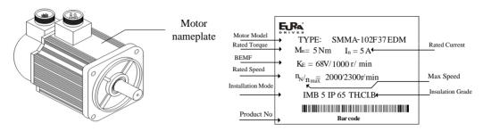
Fig 2.2.3 Servo motor nameplate (below 7.5kw)
