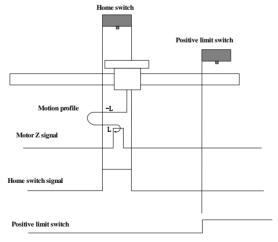
When homing starts and ORGP=1, the motor directly starts homing in negative direction at low speed. The motor changes to run in positive direction at low speed after reaching the falling edge of the ORGP signal. After reaching the rising edge of the ORGP signal, the motor stops at the first motor Z signal.
