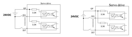
Fig 4.3.3 Passive contact interface circuit
