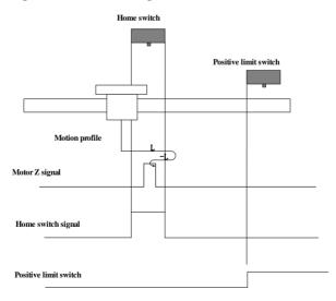
When homing starts and ORGP=1, the motor directly starts homing in positive direction at low
