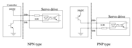
Fig 4.3.5 DI8 wiring diagram
