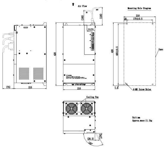
Fig 3.1.8 Servo drive structure size 6
