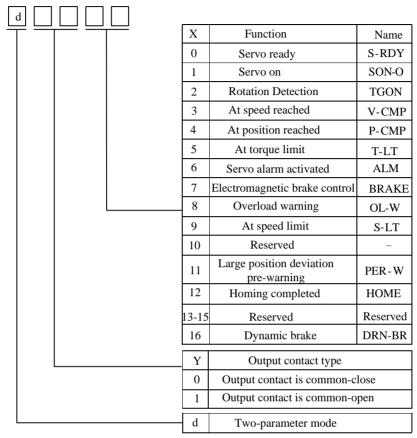
Fig 8.1.2 Programmable output terminal function
