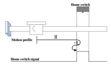
The ORGP signal is inactive initially. The motor starts homing in positive direction at high speed. If the motor does not reach the limit switch, it decelerates and changes to run in negative direction at low speed after reaching the rising edge of the ORGP signal. After reaching the falling edge of the ORGP signal, the motor stops.
