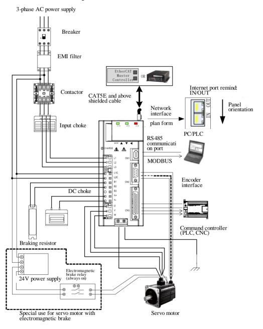
Fig 2.1.4 Composition of servo system
