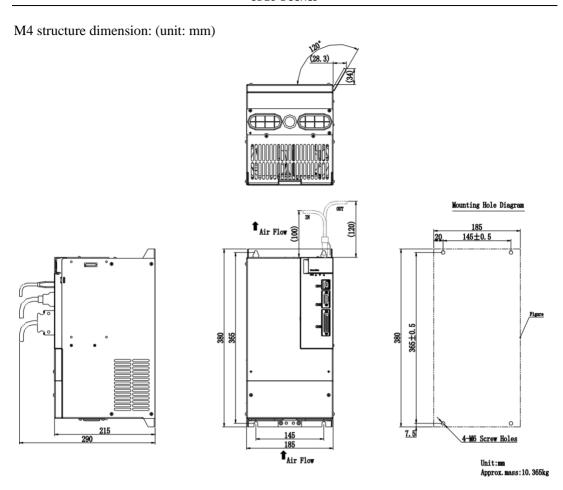
Fig 3.1.7 Servo drive structure size 5
