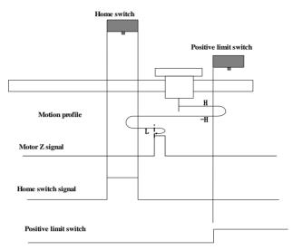
When homing starts and ORGP=0, the motor directly starts homing in positive direction at high speed. If the motor reaches the limit switch, it automatically changes to run in negative direction at high speed. After reaching the rising edge of the ORGP signal, the motor decelerates and resumes to run in positive direction at low speed. After reaching the falling edge of the ORGP signal, the motor stops at the first motor Z signal.
