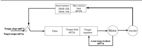
Fig 7.5.1 Block diagram for the PT mode
