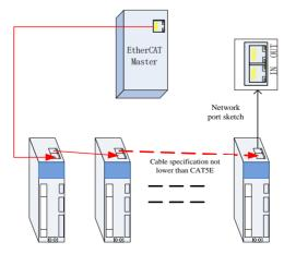
Fig 6.1.1 EtherCAT network connection sketch map
