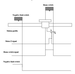
When homing starts and ORGP=1, the motor starts homing in positive direction at low speed. After reaching the falling edge of the ORGP signal, the motor changes to run in negative direction at low speed. After reaching the rising edge of the ORGP signal, the motor stops at the first motor Z signal.
