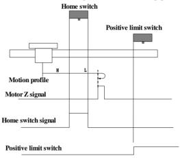
When homing starts and ORGP=0, the motor directly starts homing in positive direction at high speed. If the motor does not reach the limit switch, the motor decelerates in positive direction at low speed after reaching the rising edge of the ORGP signal. After reaching the falling edge of the ORGP signal, the motor continues running in positive direction at low speed and the motor stops at the first motor Z signal.
