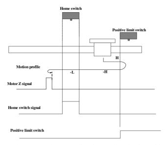
When homing starts and ORGP=0, the motor directly starts homing in positive direction at high speed. If the motor does not reach the limit switch, it automatically changes to run in negative direction at high speed. After reaching the rising edge of the ORGP signal, the motor decelerates and continues to run in negative direction at low speed. After reaching the falling edge of ORGP signal, the motor stops at first motor Z signal.
