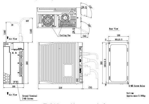
Fig 3.1.5 servo drive structure size 3
