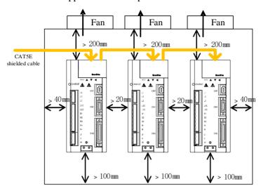
Fig 3.1.2 min installation dimension for multiple drives installed
