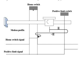
The ORGP signal is inactive initially, and the motor starts homing in positive direction at high speed. If the motor reaches the limit switch, it automatically changes to run in negative direction at high speed. After reaching the rising edge of the ORGP signal, the motor decelerates and
