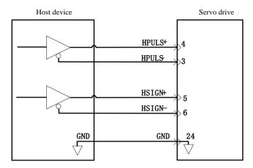
Fig 4.3.3 High-speed pulse input interface circuit
