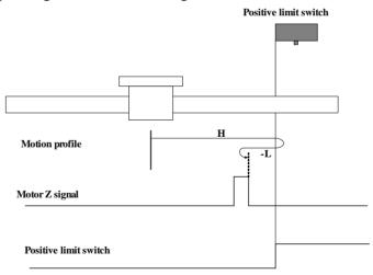
When homing starts and F-INH=0, the motor starts homing in positive direction at high speed. After reaching the rising edge of the F-INH signal, the motor decelerates and changes to run in negative direction at low speed. After reaching the falling edge of the F-INH signal, the motor stops at the first motor Z signal.
