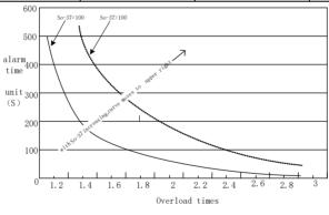
Fig 7.10.1Motor overload curve and alarm time curve graph
