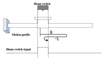
The ORGP signal is active initially. The motor starts homing in positive direction at high speed. After reaching the falling edge of the ORGP signal, the motor decelerates and changes to run in negative direction at low speed. After reaching the rising edge of the ORGP signal, the motor stops.
