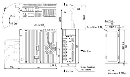
Fig 3.1.4 servo drive structure size 2
