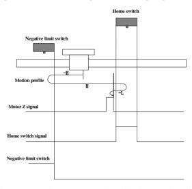
When homing starts and ORGP=0, the motor starts homing in negative direction at high speed. If the motor reaches the limit switch, the motor automatically changes the direction and runs in positive direction at high speed. The motor decelerates and runs in negative direction at low speed after reaching the rising edge of the ORGP signal. After reaching the falling edge of the ORGP signal, the motor stops at the first motor Z signal.
