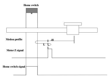
When homing starts and ORGP=0, the motor directly starts homing in negative direction at high speed. After reaching the rising edge of the ORGP signal, the motor decelerates and changes to run in positive direction at low speed. After reaching the falling edge of the ORGP signal, the motor stops at the first motor Z signal.
