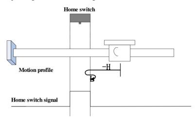
The ORGP signal is inactive initially. The motor starts homing in negative direction at high speed. If the motor does not reach the limit switch, it decelerates and changes to run in positive
