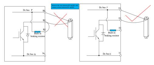
Fig 7-1-11 Wiring of braking resistor
