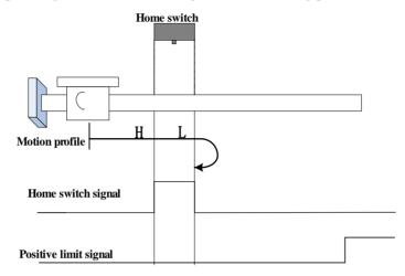
The ORGP signal is inactive initially. The motor starts homing in positive direction at high speed. If the motor does not reach the limit switch, it decelerates and continues to run in positive direction at low speed after reaching the rising edge of the ORGP signal. After reaching the falling edge of the ORGP signal, the motor stops.
