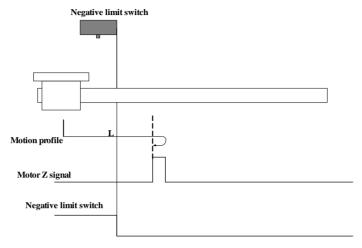
When homing starts and R-INH=1, the motor directly starts homing in positive direction at low speed. After reaching the falling edge of the R-INH signal, motor stops at first motor Z signal.
