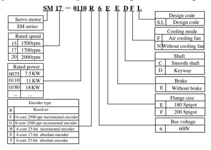
Fig 2.2.2 Servo motor naming rule (for 180 spigot and 250 spigot motor)
