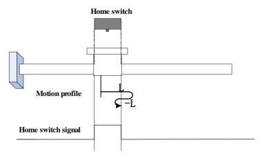
The ORGP signal is active initially, and motor directly starts homing in positive direction at low speed. After reaching the falling edge of the ORGP signal, the motor changes to run in negative direction at low speed. After reaching the rising edge of the ORGP signal, the motor stops.
