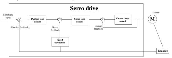
Based on the command modes and running characteristics, servo drives supports three running mode, position control, speed control and torque control.
