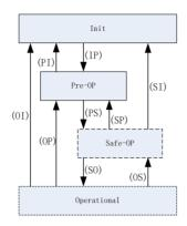
Fig 6.1.4 EtherCAT state machine
