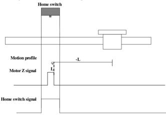
When homing starts and ORGP=0, the motor directly starts homing in positive direction at low speed. After reaching the rising edge of the ORGP signal, the motor stops at the first motor Z signal.
