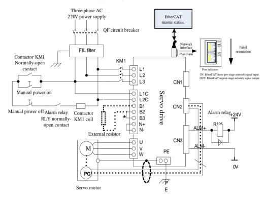
Fig 4.1.7 Typical wiring of 220V servo main circuit
