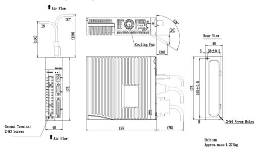
Fig 3.1.3 Servo drive structure size 1
