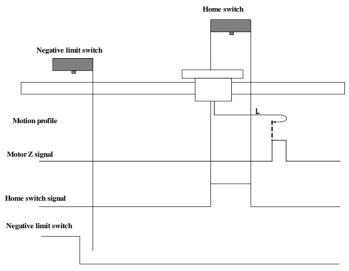
When homing starts and ORGP=1, and the motor directly starts homing in positive direction at low speed. After reaching the falling edge of the ORGP signal, the motor stops at the first motor Z signal.
