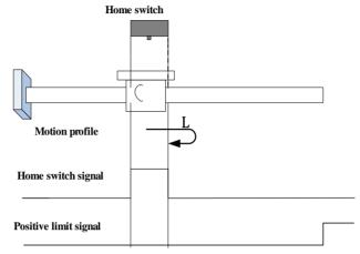
The ORGP signal is active initially, and the motor directly starts homing in positive direction at low speed.
