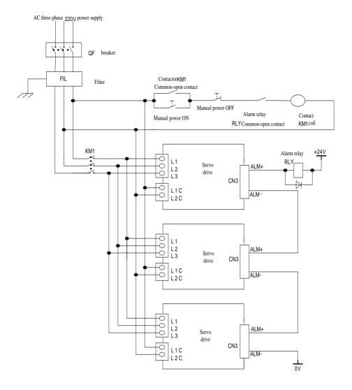
Fig 4.3.13 220V multiple online wiring
