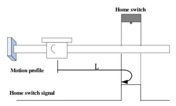
The ORGP signal is inactive initially, and the motor starts homing in positive direction at low speed.
