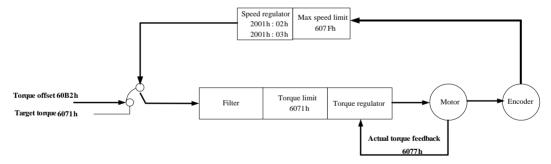
Fig 7.8.1 Configuration block diagram for CST mode
