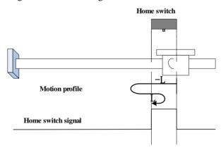
The ORGP signal is active initially, and the motor directly starts homing in negative direction at
