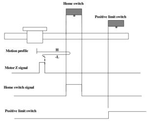
When homing starts and ORGP=0, the motor directly starts homing in positive direction at high speed. If the motor does not reach the limit switch, it decelerates and changes to run in negative direction at low speed after reaching rising edge of the ORGP signal. After reaching falling edge of the ORGP signal, the motor stops at first motor Z signal.
