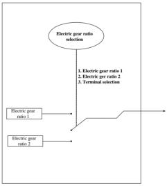
When 2003h-05h and 6091h-01h are not 0, electronic gear ratio equals to 2003h-05h/2003h-06h (or 6091h-01h/6091h-02h). If 2003h-05h or (6091h-01h)=0, pulse numbers of motor rotating a rotation is controlled by 2003h-06h or (6091h-02h).
