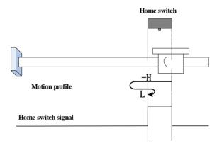
The ORGP signal is active initially. The motor starts homing in negative direction at high speed. After reaching the falling edge of the ORGP signal, the motor decelerates and changes to run in positive direction at low speed.
