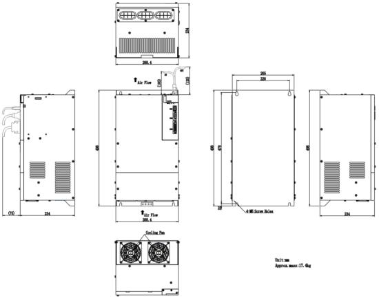
Fig 3.1.9 Servo drive structure size 7
