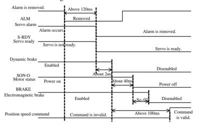
Fig 7-1-8 sequence control after resetting servo drive
