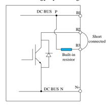
Fig 7-1-10 Wiring of energy consumption braking
