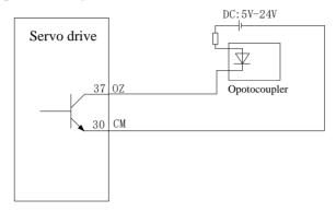
Fig 4.3.11 collector OZ signal interface circuit
