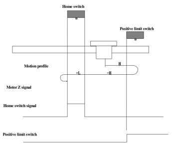
The ORGP signal is inactive initially, and the motor starts homing in positive direction at high speed. If the motor reaches the limit switch, it automatically changes to run in negative direction at high speed. After reaching the rising edge of the ORGP signal, the motor decelerates and
