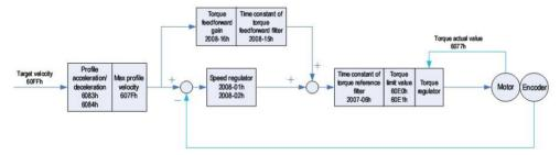
Fig 7.4.1 Block diagram for the PV mode
