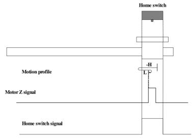
When homing starts and ORGP=1, the motor directly starts homing in negative direction at high speed. After reaching the falling edge of the ORGP signal, the motor decelerates and changes to run in negative direction at low speed. After reaching the rising edge of the ORGP signal, the motor stops at the first motor Z signal.
