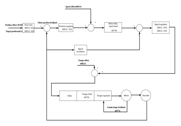
Fig 7.6.1 Configuration block diagram for CSP mode
