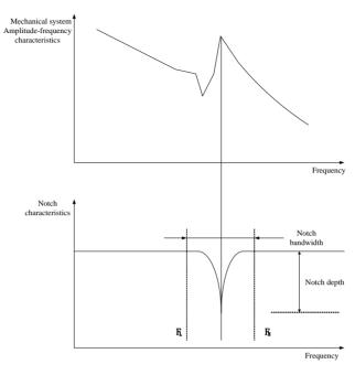
Fig 7.4.1Inhibition principle of notch filter
