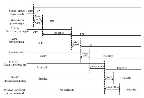
Fig 7.1.6 Time sequence at power-on
