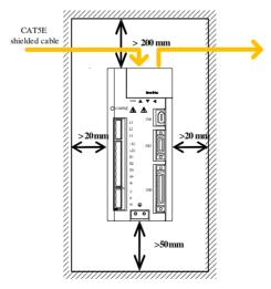
Fig 3.1.1 typical min installation dimension
