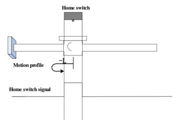
The ORGP signal is active initially, and the motor directly starts homing in negative direction at low speed.
