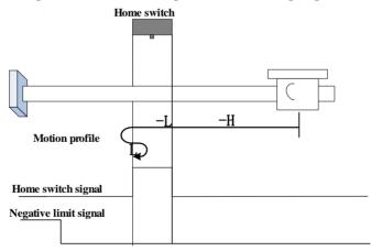
The ORGP signal is inactive initially, and the motor starts homing in negative direction at high speed. If the motor does not reach the limit switch, it decelerates and continues to run in negative direction at low speed after reaching the rising edge of the ORGP signal. After reaching the falling edge of the ORGP signal, the motor changes to run in positive direction at low speed, and stops at the rising edge of the ORGP signal.
