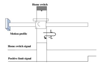
The ORGP signal is active initially, and the motor directly starts homing in positive direction at low speed.
