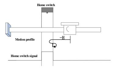
The ORGP signal is inactive initially. The motor starts homing in negative direction at high speed. After reaching the rising edge of the ORGP signal, the motor decelerates and changes to run in positive direction at low speed. After reaching the falling edge of the ORGP signal, the motor stops.
