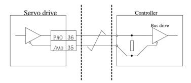
Fig 4.3.10 differential chip interface circuit of encoder frequency-dividing output
