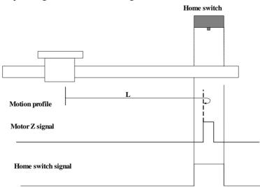
When homing starts and ORGP=0, the motor directly starts homing in positive direction at low
