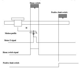
When homing starts and ORGP=0, the motor directly starts homing in positive direction at high speed. If the motor does not reach the limit switch, it decelerates and changes to run in negative direction at low speed after reaching the rising edge of the ORGP signal. After reaching the falling edge of the ORGP signal, the motor changes to run in positive direction at low speed. After reaching the rising edge of the ORGP signal, the motor stops at the first motor Z signal.
