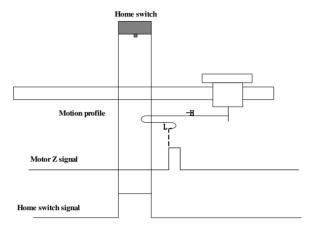
When homing starts and ORGP=0, the motor directly starts homing in negative direction at high speed. If the motor does not reach the limit switch, the motor decelerates and runs in negative direction at low speed after reaching the rising edge of the ORGP signal. After reaching the falling edge of ORGP signal, the motor stops at first motor Z signal.
