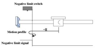
The R-INH signal is inactive initially. The motor starts homing in negative direction at high speed. After reaching the rising edge of the R-INH signal, the motor decelerates and changes to run in positive direction at low speed. After reaching the falling edge of the R-INH signal, the motor stops.
