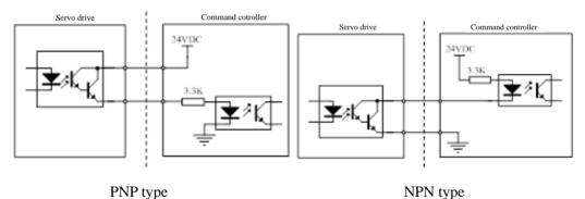
Fig 4.3.8 photoelectric coupler output interface circuit
