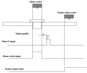
When homing starts and ORGP=1, and the motor directly starts homing in positive direction at low speed. After reaching the falling edge of the ORGP signal, the motor stops at the first motor Z signal.
