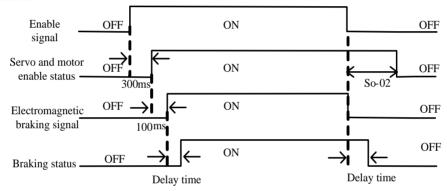
Fig 7-1-3 Electromagnetic brake sequence diagram
