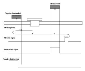
When homing starts and ORGP=0, the motor directly starts homing in negative direction at high speed. If the motor reaches the limit switch, the motor automatically changes to run in positive direction at high speed. After reaching the rising edge of the ORGP signal, the motor decelerates and continues to run in negative direction at low speed. After reaching the falling edge of the
