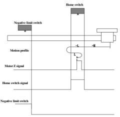
When homing starts and ORGP=0, the motor starts homing in negative direction at high speed. If the motor does not reach the limit switch, the motor decelerates and runs in negative direction at low speed after reaching the rising edge of the ORGP signal. After reaching the falling edge of the ORGP signal, the motor changes to run in positive direction at low speed. After reaching the rising edge of the ORGP signal, the motor stops at the first motor Z signal.
