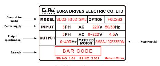
Fig 2.1.2 Servo drive nameplate
