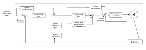
Fig 9.3.1 Servo drive internal frame diagram
