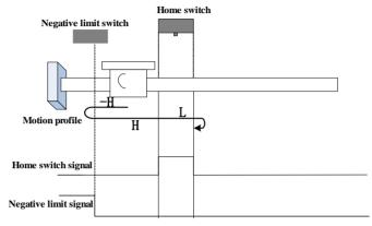
The ORGP signal is inactive initially, and the motor starts homing in negative direction at high speed. If the motor reaches the limit switch, it automatically changes to run in positive direction at high speed. After reaching the rising edge of the ORGP signal, the motor decelerates and continues to run in positive direction at low speed. After reaching the falling edge of the ORGP signal, the motor stops.
