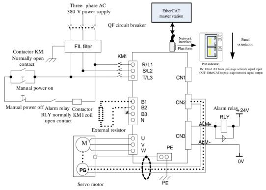
Fig 4.1.8 Typical wiring of 380V servo main circuit
