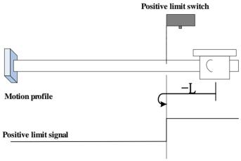
The F-INH signal is active initially, and the motor directly starts homing in negative direction at low speed.
