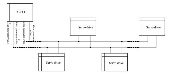
Fig 6.4.1 Field bus connection
