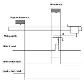
When homing starts and ORGP=0, the motor starts homing in negative direction at high speed. If the motor does not reach the limit switch, the motor decelerates and changes to run in positive direction at low speed after reaching the rising edge of the ORGP signal. After reaching the falling edge of the ORGP signal, the motor changes to run in negative direction at low speed. After reaching the rising edge of the ORGP signal, the motor stops at the first motor Z signal.
