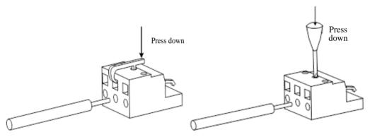
Fig 4.1.3 Main circuit terminals connection method
