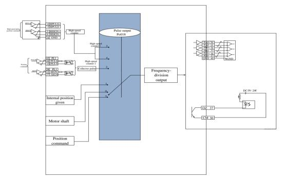
Fig 7.2.5 Frequency-division output diagram
