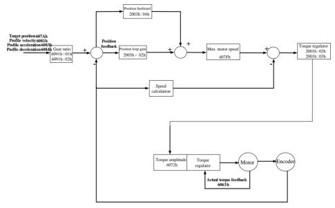
Fig 7.3.1 Block diagram for the PP mode
