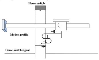
The ORGP signal is inactive initially, and the motor starts homing in negative direction at high speed. If the motor does not reach the limit switch, it decelerates and changes to run in positive direction at low speed after reaching the rising edge of the ORGP signal. After reaching the falling edge of the ORGP signal, the motor changes to run in negative direction at low speed, and stops at the rising edge of the ORGP signal.
