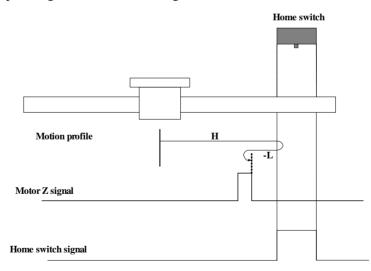
When homing starts and ORGP=0, the motor starts homing in positive direction at high speed. After reaching the rising edge of the ORGP signal, the motor decelerates and changes to run in negative direction at low speed. After reaching the falling edge of the ORGP signal, the motor
