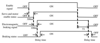
Fig 7-1-4 Electromagnetic brake sequence diagram
