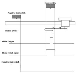
When homing starts and ORGP=0, the motor starts homing in negative direction at high speed. If the motor does not reach the limit switch, the motor decelerates and runs in negative direction at low speed after reaching the rising edge of the ORGP signal. After reaching the falling edge
