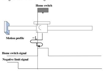
The ORGP signal is active initially, and the motor directly starts homing in negative direction at low speed.
