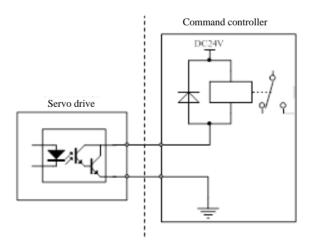
Fig 4.3.6 Relay output interface correct circuit diagram
