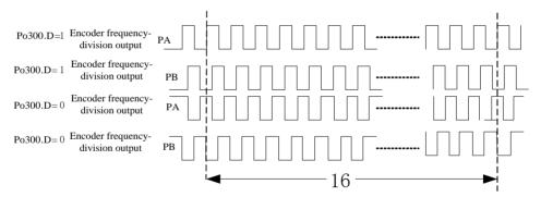
Fig 7-2-6 Encoder frequency-division output
