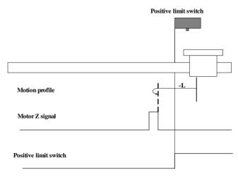
When homing starts and F-INH=1, the motor directly starts homing in positive direction at low speed. After reaching the falling edge of F-INH signal, motor stops at the first motor Z signal.
