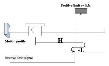
The F-INH signal is inactive initially. The motor starts homing in positive direction at high speed.
