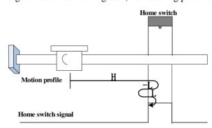
The ORGP signal is inactive initially, and the motor starts homing in positive direction at high speed.
