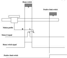
When homing starts and ORGP=0, the motor directly starts homing in positive direction at high speed. If the motor does not reach the limit switch, the motor decelerates in positive direction at low speed after reaching the rising edge of the ORGP signal. After reaching the falling edge of the ORGP signal, the motor changes to run in positive direction at low speed. After reaching the rising edge of the ORGP signal, the motor stops at the first motor Z signal.
