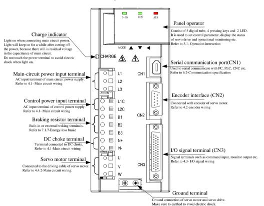
Fig 2.1.3 Composition of servo drive
