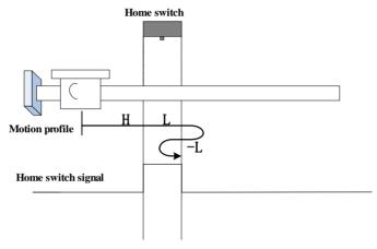
The ORGP signal is inactive initially, and the motor starts homing in positive direction at high speed. If the motor does not reach the limit switch, it decelerates and continues to run in positive direction at low speed after reaching the rising edge of the ORGP signal. After reaching the falling edge of the ORGP signal, the motor changes to run in negative direction at low speed, and stops at the rising edge of the ORGP signal.
