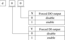
Master station can monitor DI state by reading 60FDh bit state.
