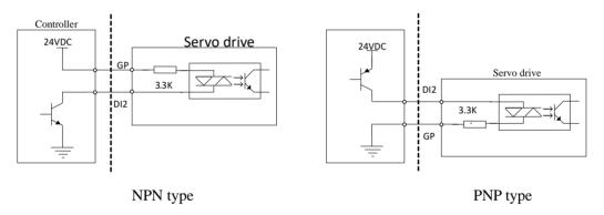
Fig 4.3.4 Active contact interface circuit
