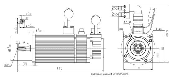
Fig 3.2.3 Servo motor installation dimension
