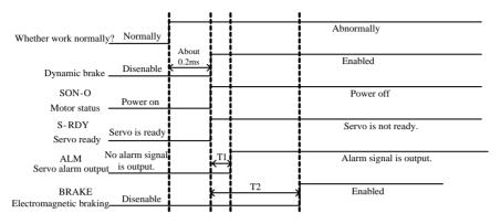
Fig 7-1-7 Sequence control of servo alarm activated
