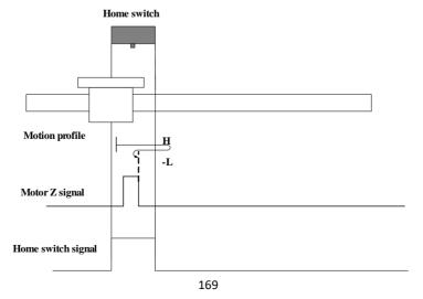
When homing starts and ORGP=1, the motor directly starts homing in positive direction at high speed. After reaching the falling edge of the ORGP signal, the motor decelerates and changes to run in negative direction at low speed. After reaching the rising edge of the ORGP signal, the motor stops at the first motor Z signal.
