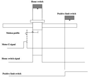
When homing starts and ORGP=1, the motor directly starts homing in negative direction at low speed. After reaching the falling edge of the ORGP signal, the motor stops at the first motor Z signal.
