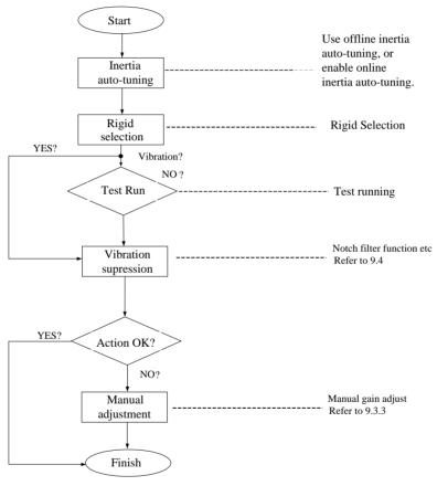
Fig 9.1.1Gain adjustment flow chart
