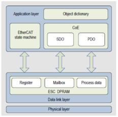
Fig 6.1.3 EtherCAT communication structure at CANopen application layer
