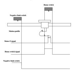
When homing starts and ORGP=1, the motor directly starts homing in positive direction at low speed. After reaching the falling edge of the ORGP signal, the motor changes to run in positive direction at low speed. After reaching the rising edge of ORGP signal, motor stops at first motor Z signal.
