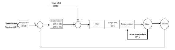
Fig 7.7.1 Configuration block diagram for CSV mode
