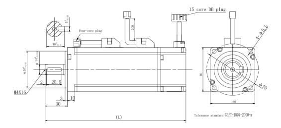
Fig 3.2.1 Motor installation dimension
