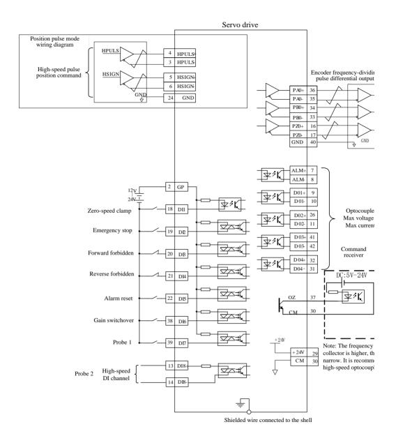
Fig 4.3.1 Wiring diagram in bus mode
