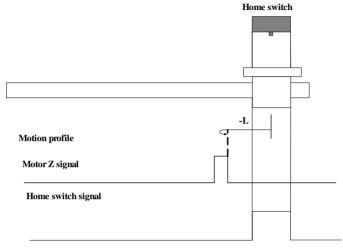
When homing starts and ORGP=1, the motor directly starts homing in positive direction at low speed. After reaching the falling edge of the ORGP signal, the motor stops at the first motor Z signal
