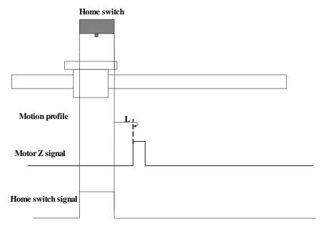
When homing starts and ORGP=1, the motor directly starts homing in positive direction at low speed. After reaching the falling edge of the ORGP signal, the motor stops at the first motor Z signal.
