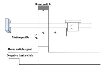
The ORGP signal is inactive initially. The motor starts homing in negative direction at high speed. If the motor does not reach the limit switch, it decelerates and continues to run in negative direction at low speed after reaching the rising edge of the ORGP signal. After reaching the falling edge of the ORGP signal, the motor stops.
