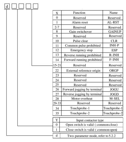
Fig 8.1.1 Programmable input terminal function
