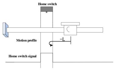
The ORGP signal is inactive initially, and the motor directly starts homing in negative direction at low speed.
