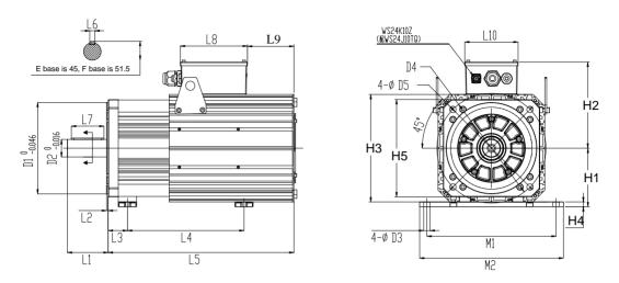
Fig 3.2.6 Servo motor installation dimension
