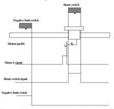
When homing starts and ORGP=1, the motor starts homing in negative direction at low speed. After reaching the falling edge of the ORGP signal, the motor stops at the first motor Z signal.
