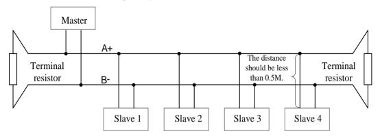
Please think over the drive capacity of PC/PLC and the distance between PC/PLC and inverter when wiring. Add a repeaters if drive capacity is not enough.
