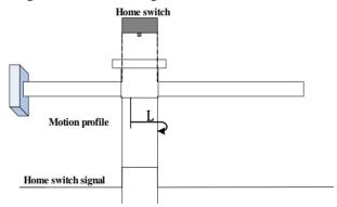
The ORGP signal is active initially, and the motor directly starts homing in positive direction at low speed.
