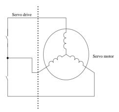
Fig 7-1-9 Dynamic braking
