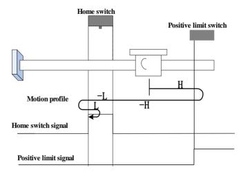
The ORGP signal is inactive initially, and the motor starts homing in positive direction at high speed.
