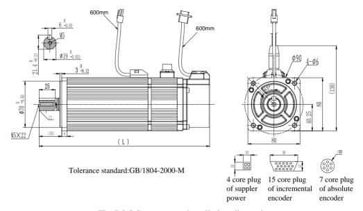
Fig 3.2.2 Servo motor installation dimension
