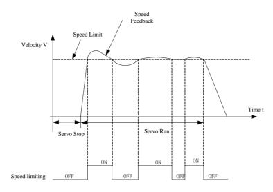
Fig 7.10.2 Output in speed limit under torque mode sketch map
