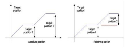
Fig 7.3.4 Difference between absolute and relative position reference
