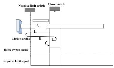
The ORGP signal is inactive initially, and the motor starts homing in negative direction at high speed. If the motor reaches the limit switch, it automatically changes to run in positive direction at high speed. After reaching the rising edge of the ORGP signal, the motor decelerates and changes to run in negative direction at low speed.
