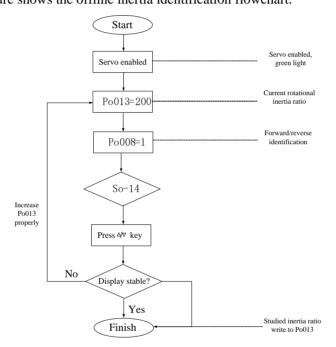
Fig 9.2.1 Offline inertia identification flowchart
