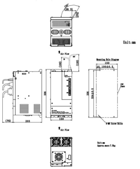
Fig 3.1.6 Servo drive structure size 4
