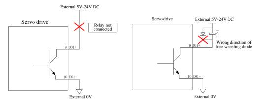
Fig 4.3.7 Wrong wiring circuit of relay output interface
