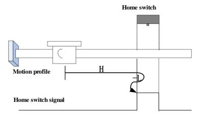
The ORGP signal is inactive initially. The motor starts homing in positive direction at high speed. After reaching the rising edge of the ORGP signal, the motor decelerates and changes to run in negative direction at low speed. After reaching the falling edge of the ORGP signal, the motor stops.
